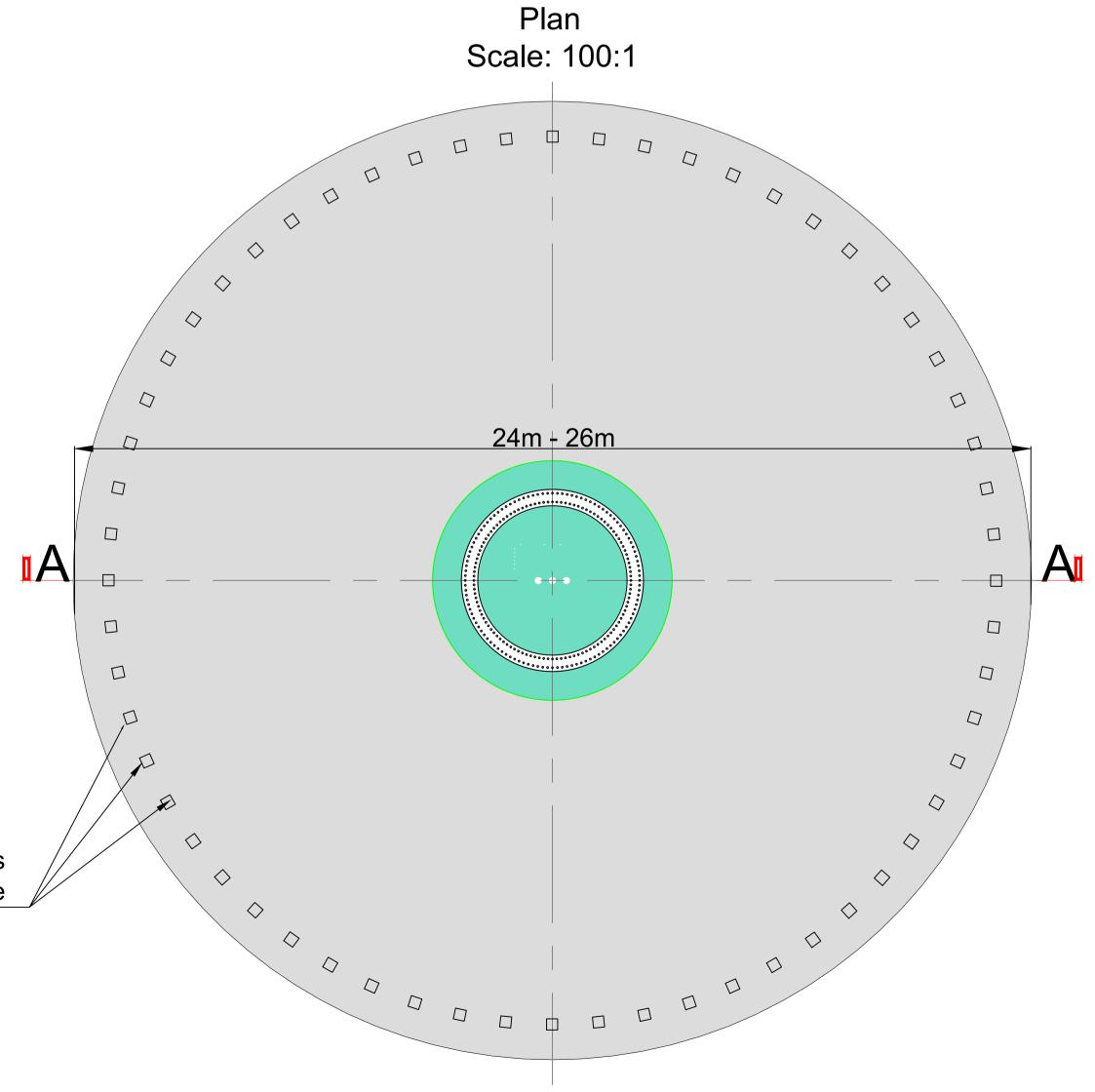
50 - 70 no. 300 x 300 mm square piles Spaced evenly around the perimeter of the turbine base
